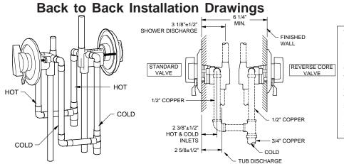
The ZURN TEMP-GARD Pressure Balancing Shower Valve is equipped with an adjustable limit stop screw. The limit stop device is to be used to limit the valve handle from being turned to undesired hot water discharge temperatures. To adjust the limit stop screw, remove handle and escutcheon, turn valve to maximum desired temperature and turn the limit stop screw until it seats
